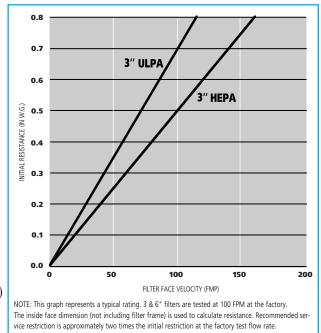
Filter Face Velocity [FPM] = Rated Flow [cu ft per min] x 144 Height of Filter [in] - (less frame) 1.50" x Width of Filter [in] - 1.50" (less frame)
